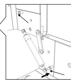
Attach the gas springs by pushing both ends to their places
